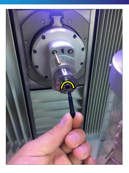
Screw in the cleaned collet chuck by hand including the tool T0 as long as the tool T0 is tighten in the collet.
